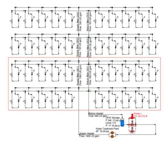
Notice the pump is red. The system was designed so that a single pump could handle four banks of tools, but not eight banks. Also notice that only one pump is currently operating.
