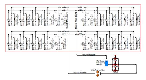
An ultra pure water system is a closed looped distribution system in which all the water going to the various tools in the plant is under positive pressure. In addition, the return piping is included so there is no dead-heading when a tool is not running. To prevent the introduction of any contamination into the system, there is a positive pressure maintained in the return header to the Ultra Pure Water (UPW) storage tank.
