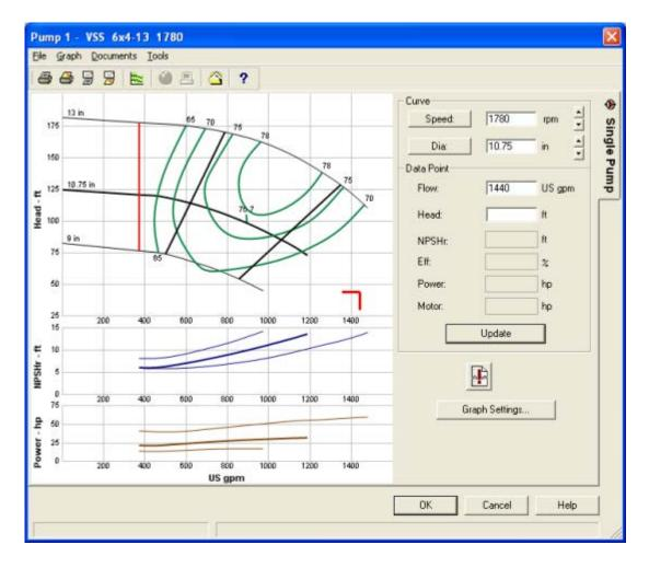
Notice the red operating point is well off the end of the graph. This pump is being stretched beyond its limits.
