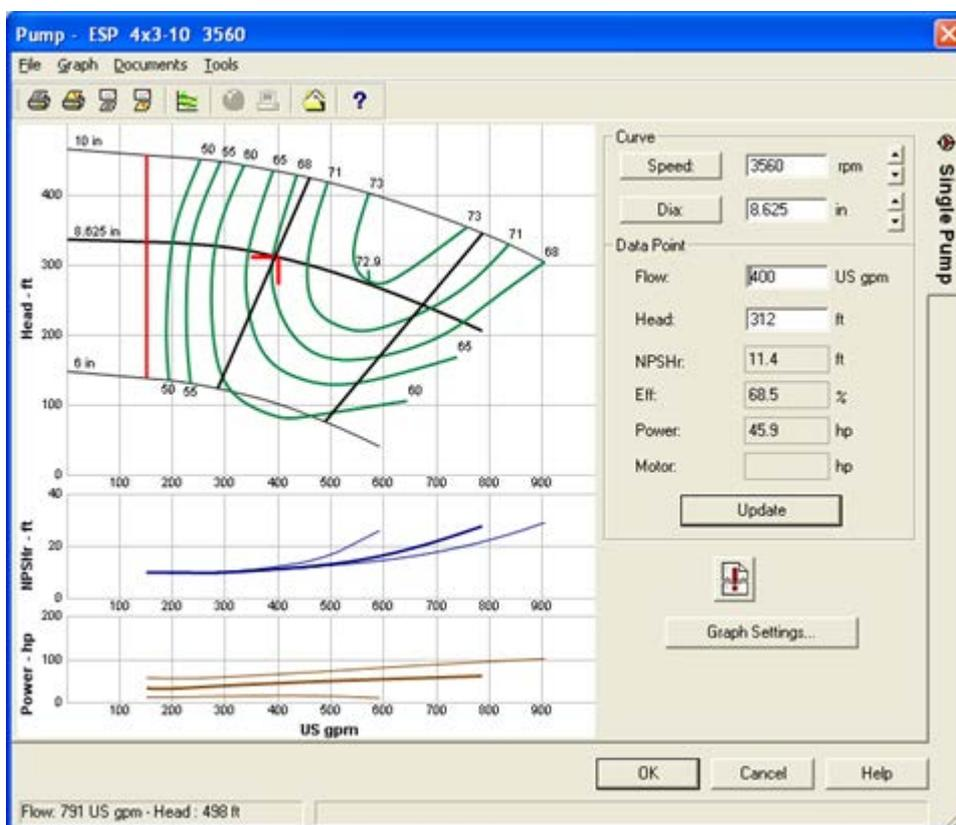
Notice the differential pressure across the FCV set to 400 gpm is over **68** psi, or a head loss of over **158** feet of fluid. In addition, the pump is running much further up on its curve with lower efficiency.
