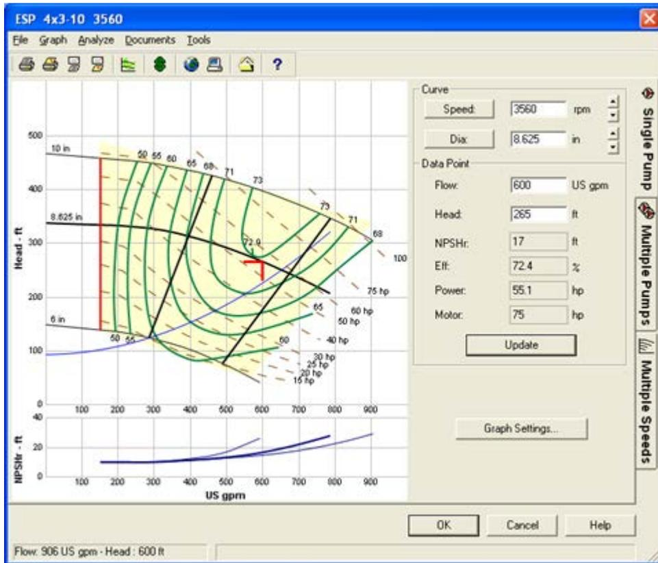
The blue line on the pump curve is the system resistance curve. To see how much it would cost to run the pump with a variable speed drive, we will do the cost analysis again with a variable speed instead of a fixed speed.
