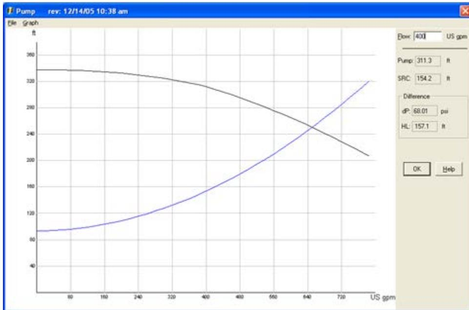
The black line is the pump curve and the blue line is the system resistance curve. You can see at 400 gpm the difference is 68.01 psi or 157.1 ft.
