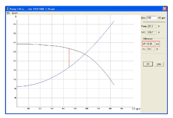
Notice the required differential pressure this time is over 35 psi.As we saw earlier, our selected globe valve drops even more (over 43 psi) to limit the flow to 450 gpm.
