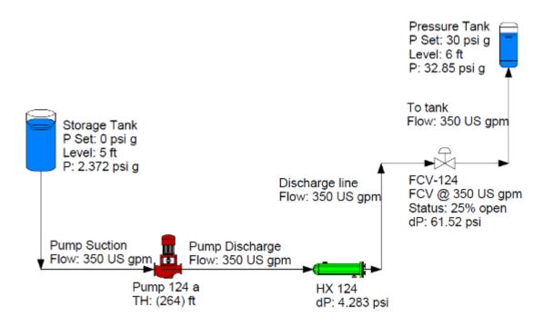
You can see that with 350 gpm going through the control valve there is a differential pressure across the valve of over 60 psi. This is a very high pressure drop for this control valve.You can also see that the valve position is 25% open.
