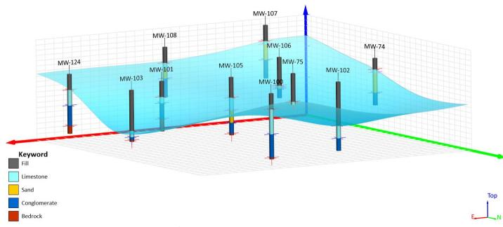
Define points of contact based on upper/lower keywords or using a query! Export those contact points to a data file for gridding and view the surface in the 3D view.
